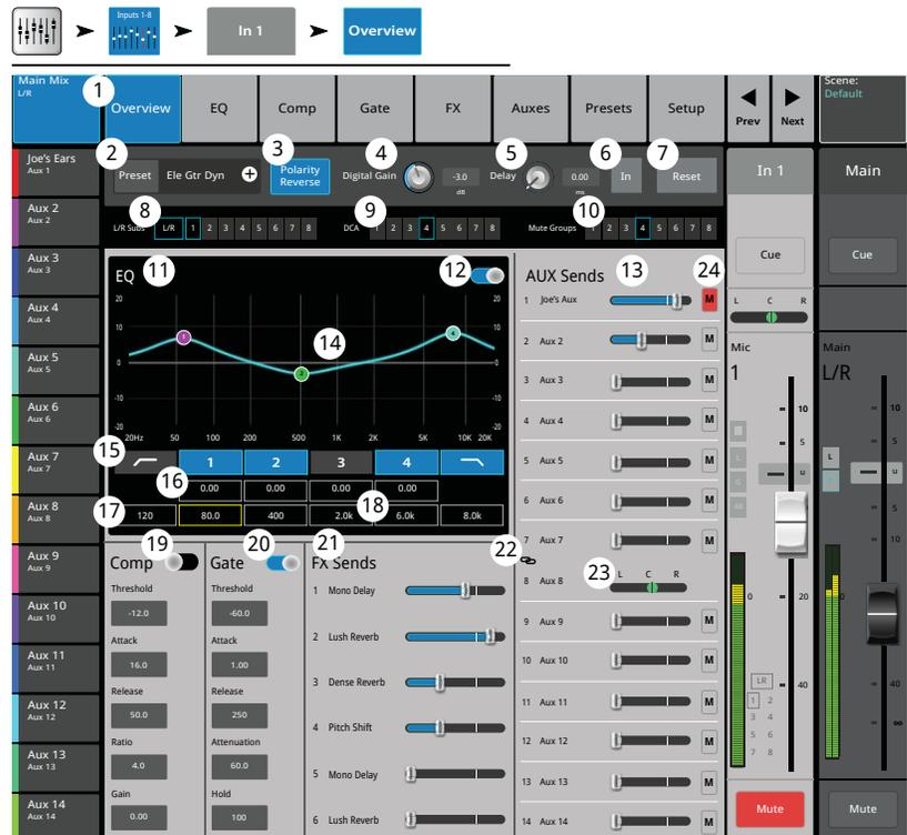
To adjust the following parameters, select the field then use the Master encoder or the up/down nudge buttons on a mobile device.
