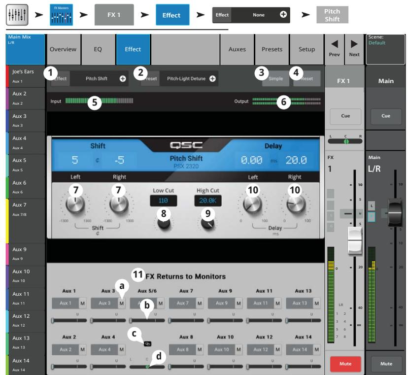
Rotating the Master Encoder will change the amount of pitch shift in half-step intervals. For finer adjustments, hold the Encoder down while adjusting.
